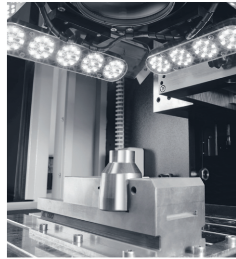
Vision system FOBA IMP: Detects the position of to-be-processed areas and parts, and aligns engraving, marking or finishing automatically and precisely as required.
